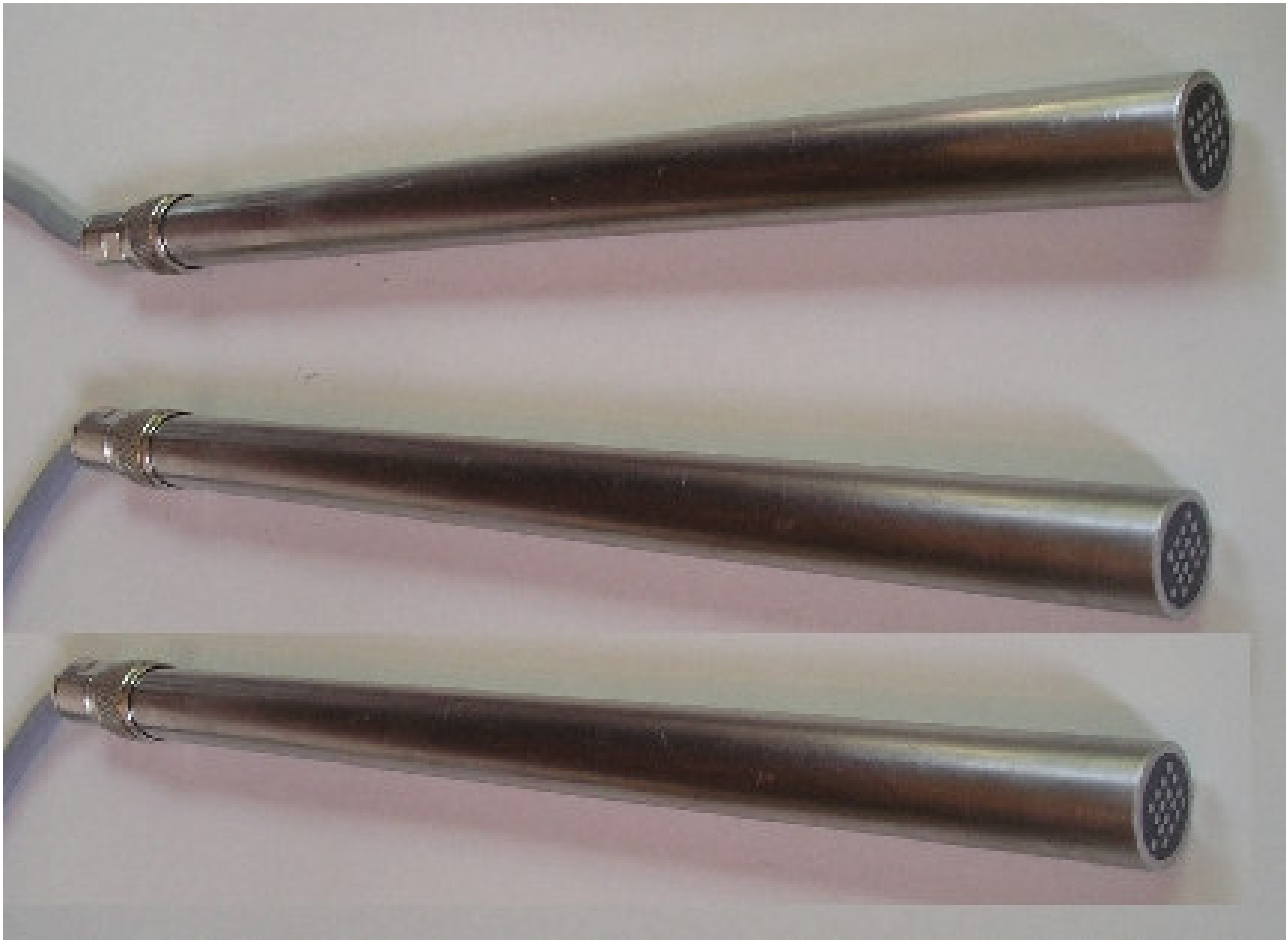
Figure 1. Typical coupled multielectrode sensors used in the experiment.
