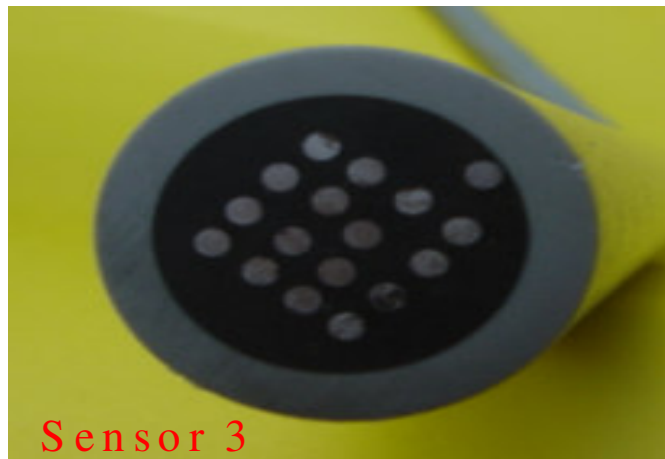
Figure 8. Appearances of the electrodes of sensors after the monitoring period. Sensor #1 electrodes were cathodically protected. Sensor #2 electrodes were anodically polarized except the shiny one that had a faulty connection (at row 3 and column 2). Sensor #3 electrodes were maintained near the free corrosion potential. The electrode outside the 4 by 4 matrix in each sensor was used as a position locator and was not part of the sensing electrodes.
