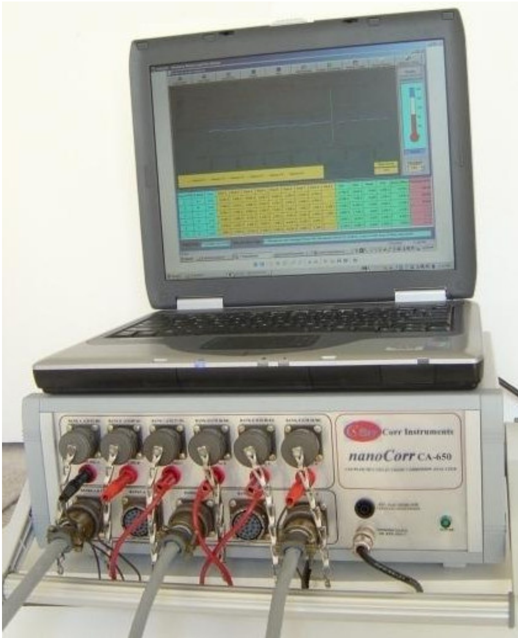
Figure 2. Coupled multielectrode corrosion analyzer system used in the experiment.
