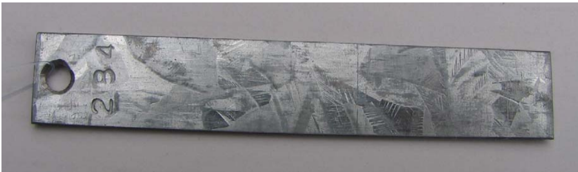
Figure V - Galvanized Coupon # 234 exposed 60 days in ZLD Tower Water Treated with TTA Supplement to Silica Inhibitor
