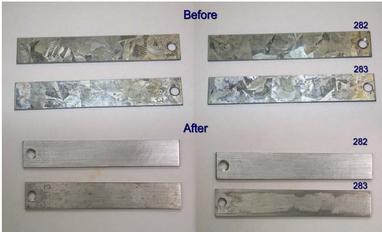
Figure IV – Galvanized coupon #283 exposed to ZLD Tower water for 60 days and #282 unexposed before and after acid strip of galvanized coating. (Note: mm/yr= mpy/39.4)
