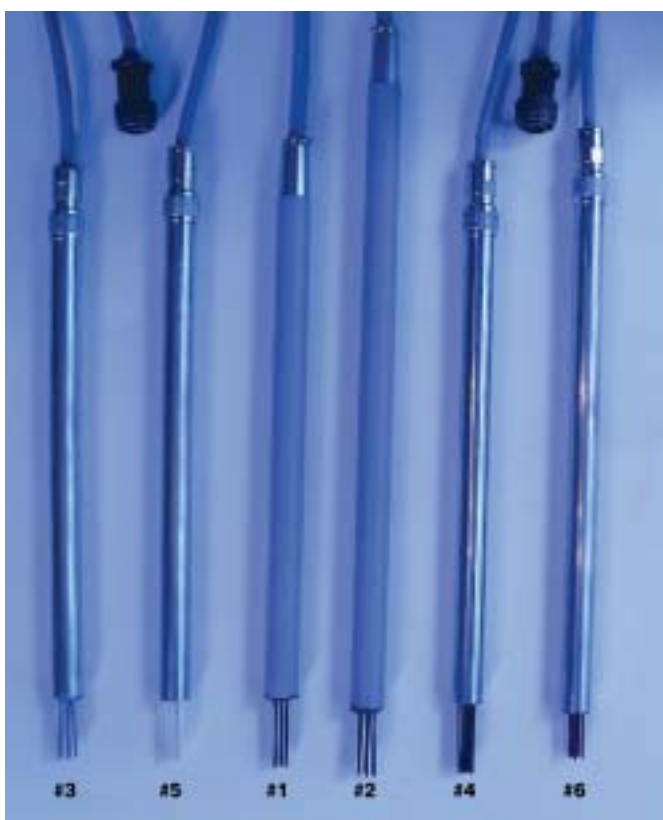
Coupled multielectrode sensors painted with different coatings for the experiment.
