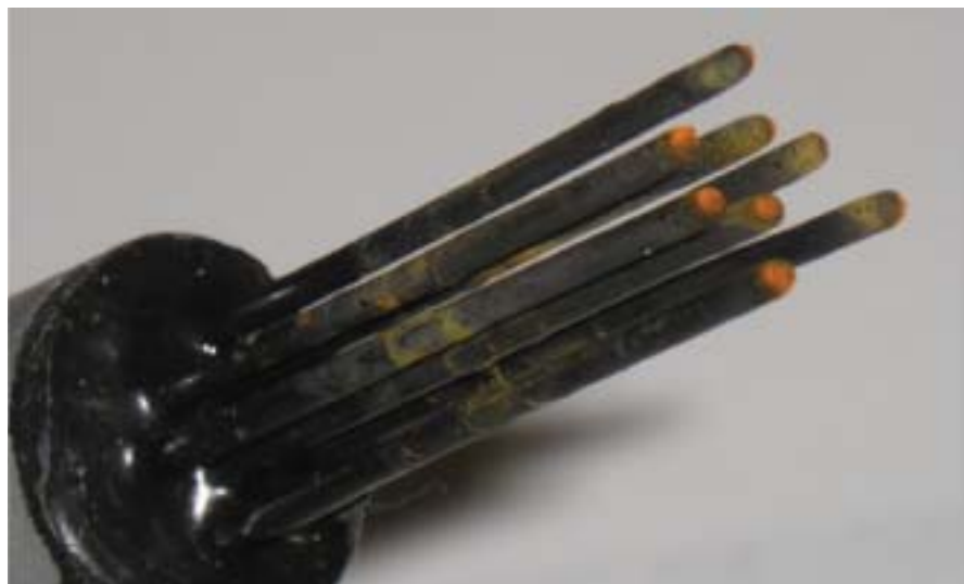
Appearances of Sensor 2 electrodes after 7 days of immersion in simulated seawater. Coatings at the tips of all electrodes contained initial defects prior to the test. The tips of the electrodes had rusted after 7 days and were severely corroded after 17 days of immersion.
