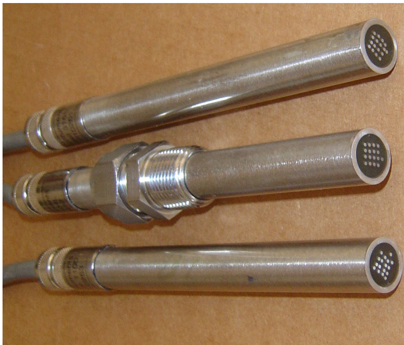
Figure 2. Typical coupled multielectrode array sensor probes.
